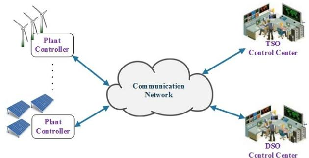
Fig. 1. Communication architecture where several plant controllers are shown communicating with control centers at different levels
