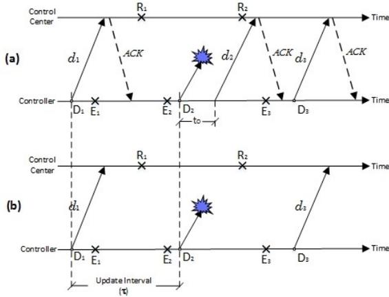
Fig. 3. Message sequence diagram showing proactive, periodic update of information with an information mismatch case scenario for (a) TCP and (b) UDP
