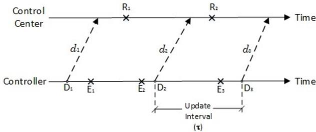
Fig. 2. Message sequence diagram showing proactive, periodic update of information with a mismatch case scenario
