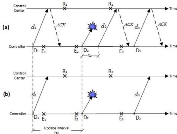
Fig. 3. Message sequence diagram showing proactive, periodic update of information with an information mismatch case scenario for (a) TCP and (b) UDP
