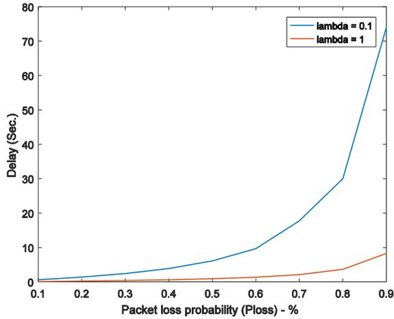
Fig. 7. Trade-off between packet-loss and end-to-end delay for a given propagation delay at minimum and maximum event rates (lambda).
