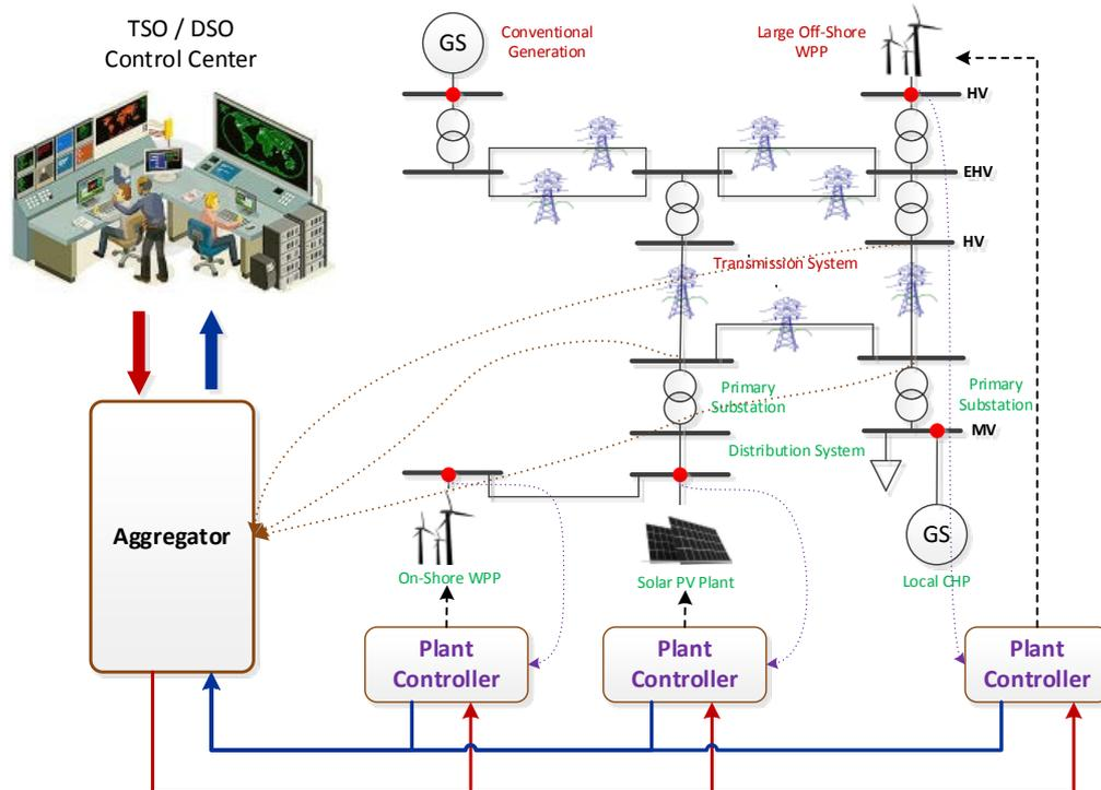
Figure 7: Sketch map of the aggregator control architecture.
