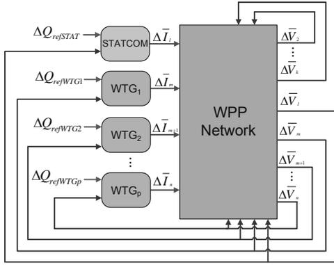
Figure 4. Functional diagram of wind power plant model used for the state-space representation.
