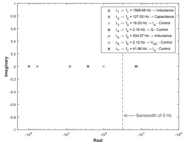
Figure 3. Eigenvalue spectrum for the WT state-space model.
