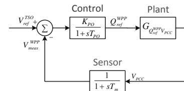
Figure 9. Control architecture used for AVR tuning
