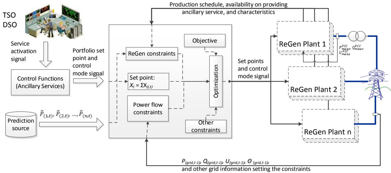
Figure 1. Input and output signals of dispatch process
