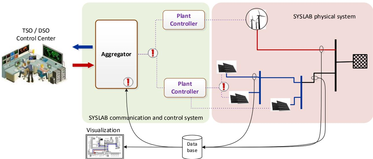
Figure 9. Control architecture of SYSLAB experiment
