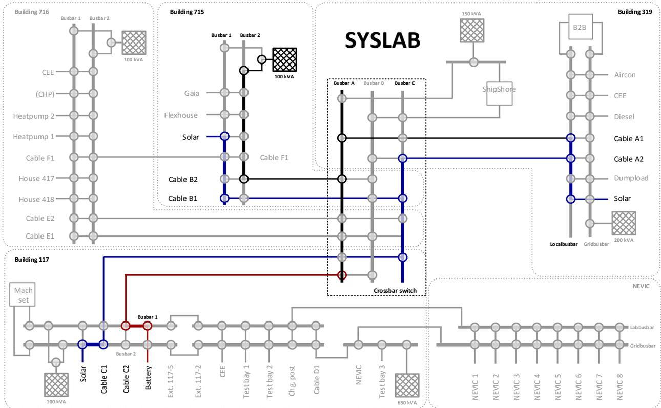
Figure 8. Physical layout of SYSLAB experiment
