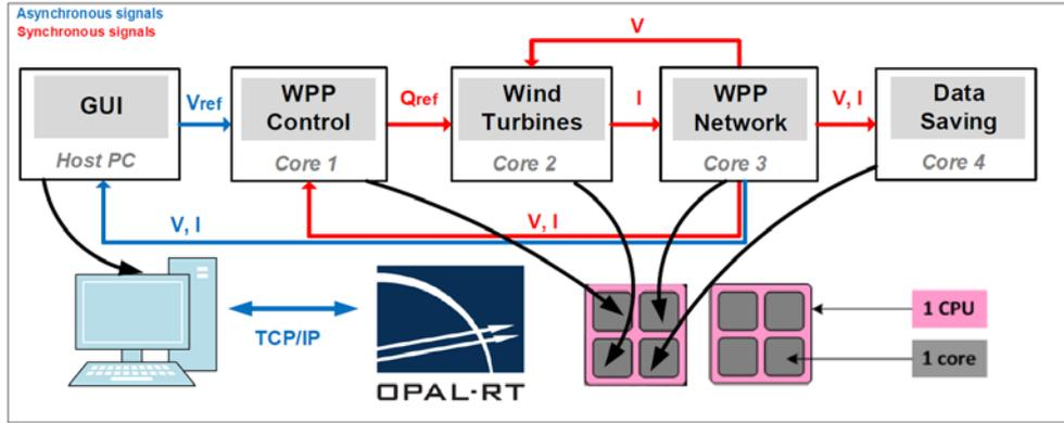
Fig. 4 Wind Power Plant Voltage Control - Implementation on *Real-Time Simulator*
