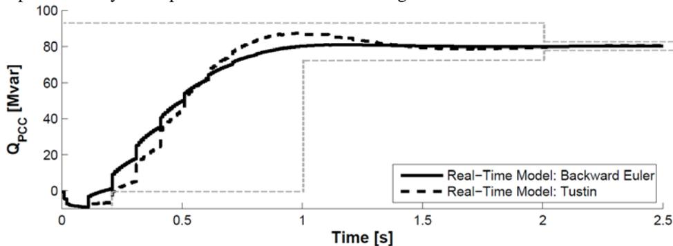
Fig. 5 Reactive power response for a grid voltage disturbance for different discretization methods
