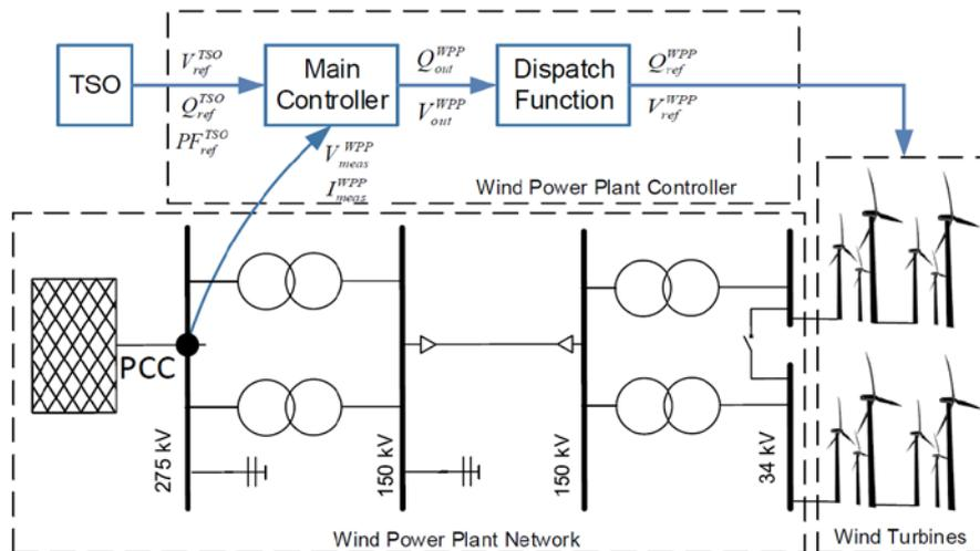
Fig. 1 Overview Wind Power Plant Voltage Control Architecture
