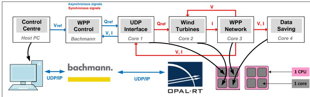
Fig. 6: Wind Power Plant Voltage Control - RT-HIL Implementation
