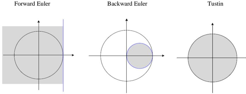
Fig. 3 Possible regions for discrete approximation methods in z-plane [9]
