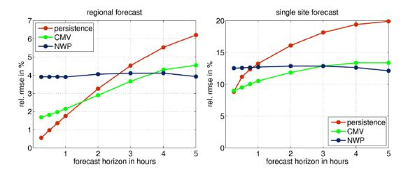
Figure 6: Performance of solar-PV prediction systems German average (left) and single site (right) [9]
