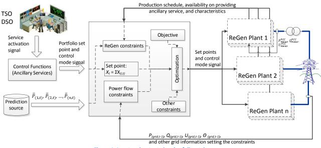
Figure 1. Input and output signals of dispatch process
