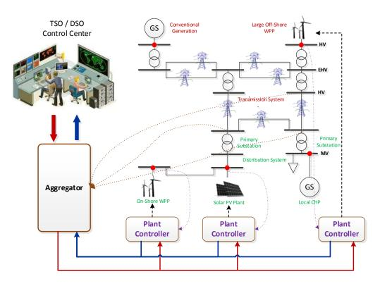
Figure 7: Sketch map of the aggregator control architecture.
