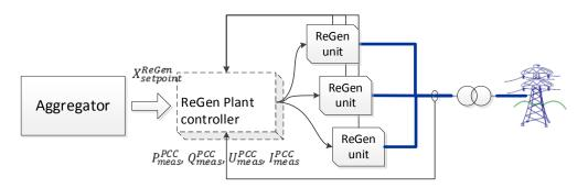
Figure 2. Plant level control diagram
