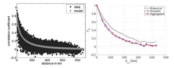
Figure 4: Correlation coefficient of forecast errors between two stations as a function of distance: solar forecast errors in Germany (left), [6] and wind forecast errors in Denmark (right), [7]
