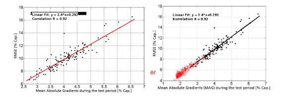
Figure 3: Correlation between RSME and MAG for a single wind power plant (left) and clusters of wind power plants (right) [5].
