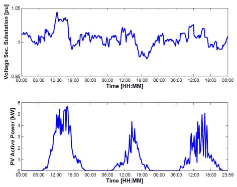
Figure 1: Voltage profile at secondary substation and power profile of one PV system (15 min values)
