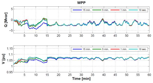
Figure 70: Q and V of WPP over one hour for various update rates Ts for voltage setpoint and grid voltage of  $V_{grid} = 1.00 \, pu$
