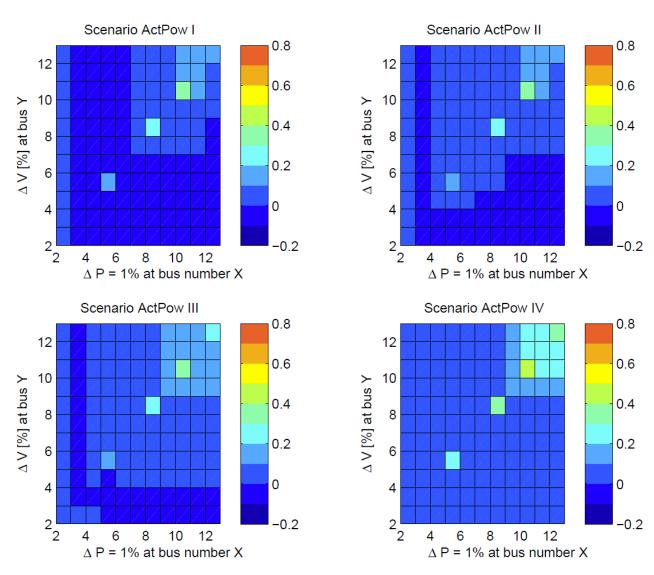
Figure 20:  $\delta V/\delta P$  sensitivity for various operational points of ReGen plants and external grid voltage  $V_{EG} = 1 pu$
