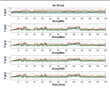
Figure 87: Voltage profile at all system busses for various droop settings and  $V_{grid}=1.05~pu$
