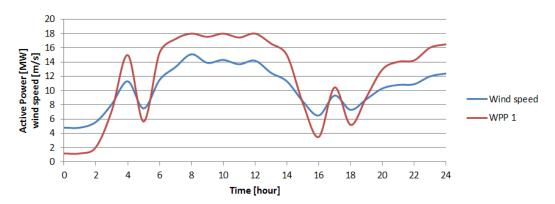
Figure 7: Exemplary daily profile of wind speed and power output of WPP with rated power of 18 MW [9]
