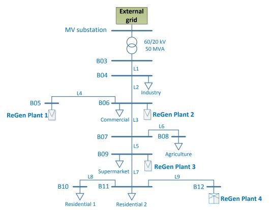
Figure 19: Structure of MV Benchmark Grid
