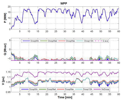
Figure 50: P, Q, V of WPP over one hour for different droop settings and grid voltage of  $V_{grid}=1.05~pu$
