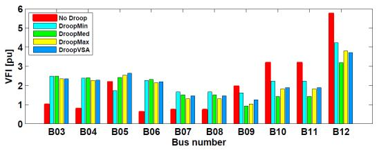
Figure 46: VFI for all MV busses and various droop settings and grid voltage of  $V_{arid} = 1.00 \, pu$
