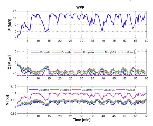
Figure 44: P, Q, V of WPP over one hour for different droop settings and grid voltage of  $V_{grid}=1.\,00\,pu$
