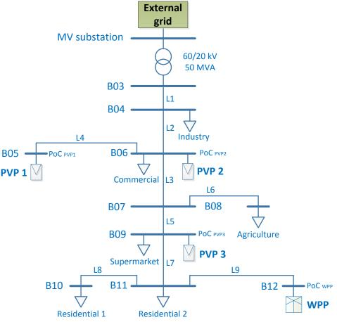
Figure 6: MV Benchmark distribution grid with ReGen plants
