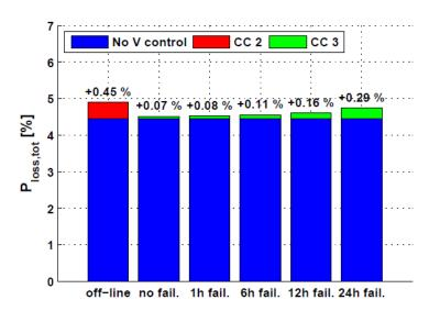
Figure 82: Power losses for various durations of communication failure for updating the voltage setpoints
