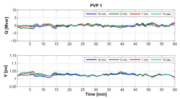
Figure 67: Q and V of PVP 1 over one hour for various update rates Ts for voltage setpoint and grid voltage of  $V_{grid} = 1.00 \ pu$
