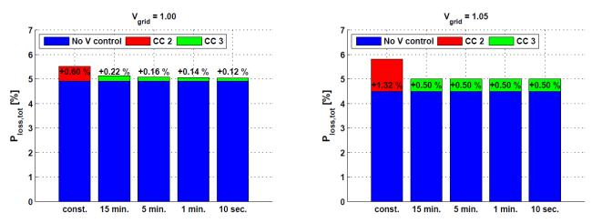
Figure 66: Power losses for various update rates Ts of voltage setpoint (left:  $V_{arid} = 1.00 pu$ , right:  $V_{arid} = 1.05 pu$ )
