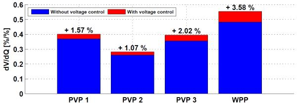
Figure 62: Diagonal elements of  $\delta V/\delta Q$  sensitivity matrix for PoC of ReGen plants - without and with voltage control
