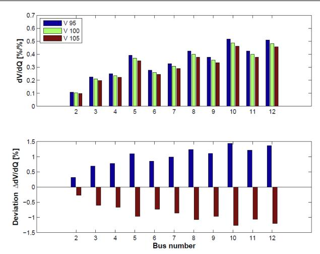
Figure 26: Diagonal elements of δV/δQ sensitivity matrix for various operational points of external grid
