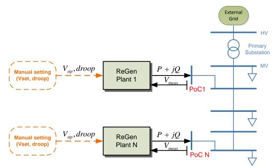
Figure 35: Scheme of control concept 1 – Manual Droop Setting
