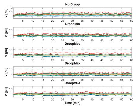
Figure 86: Voltage profile at all system busses for various droop settings and  $V_{arid} = 1.00 \, pu$
