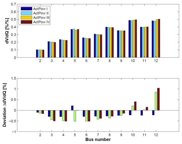
Figure 25: Diagonal elements of  $\delta V/\delta Q$  sensitivity matrix for various operational points of ReGen plants
