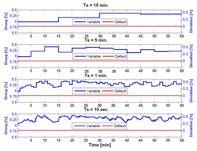
Figure 64: Default and variable voltage droop value for the WPP dependent on the update rate Ts
