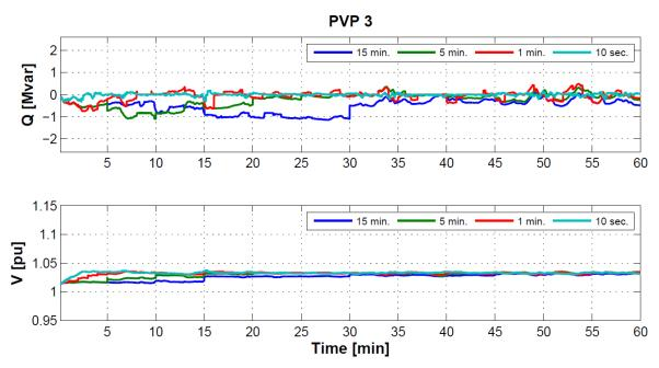
Figure 69: Q and V of PVP 3 over one hour for various update rates Ts for voltage setpoint and grid voltage of  $V_{grid} = 1.00 \ pu$
