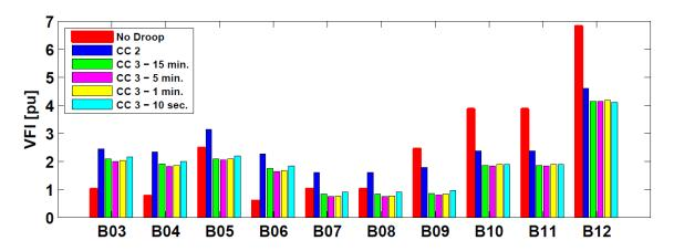
Figure 73: VFI for all MV busses and various various update rates for the voltage setpoint and grid voltage of  $V_{grid} = 1.05 \ pu$
