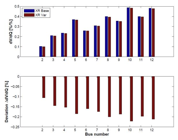
Figure 29: Diagonal elements of  $\delta V/\delta Q$  sensitivity matrix for different X/R ratios
