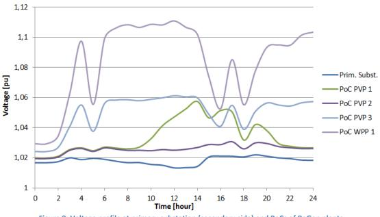
Figure 9: Voltage profile at primary substation (secondary side) and PoCs of ReGen plants
