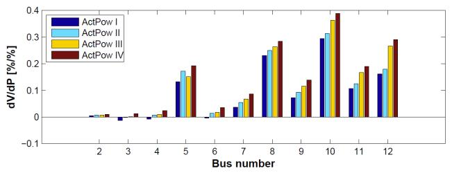
Figure 22: Diagonal elements of δV/δP sensitivity matrix for various operational points of ReGen plants
