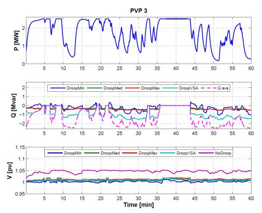
Figure 43: P, Q, V of PVP 3 over one hour for different droop settings and grid voltage of  $V_{grid}=$  1.00 pu
