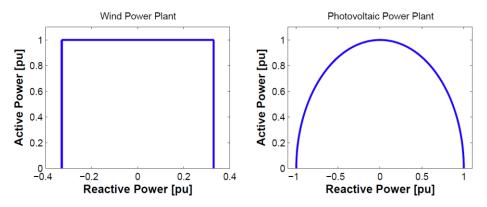
Figure 10: Reactive Power Capability charts for wind power and photovoltaic power plants [17] [18] [19]
