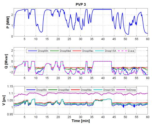
Figure 49: P, Q, V of PVP 3 over one hour for different droop settings and grid voltage of  $V_{grid}=$  1.05 pu
