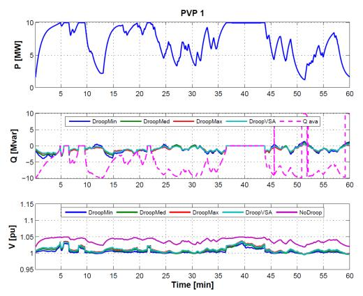
Figure 41: P, Q, V of PVP 1 over one hour for different droop settings and grid voltage of  $V_{grid}=$  1.00 pu
