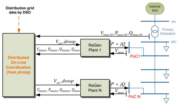
Figure 38: Scheme of control concept 3 - Distributed On-Line Coordination
