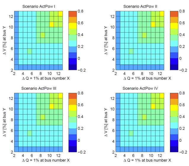
Figure 23: δV/δQ sensitivity for various operational points of ReGen plants
