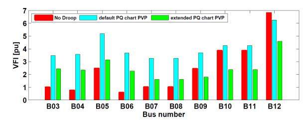
Figure 60: VFI for all MV busses and various PQ charts of PVP and grid voltage of  $V_{grid} = 1.05 \ pu$
