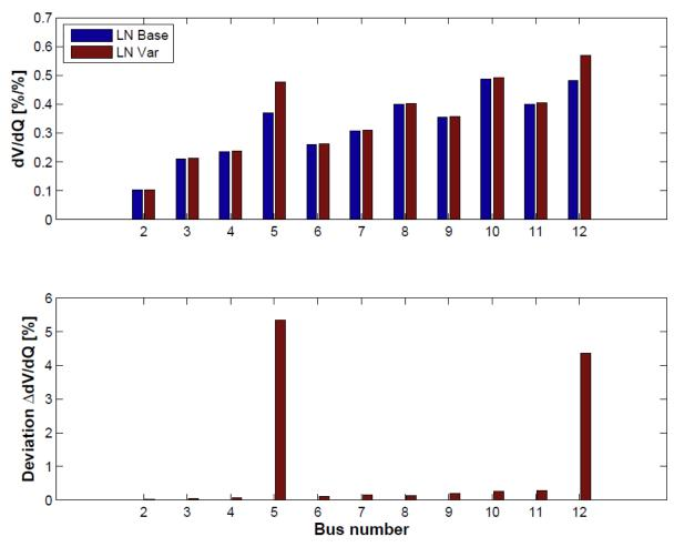
Figure 27: Diagonal elements of  $\delta V/\delta Q$  sensitivity matrix for different line lengths
