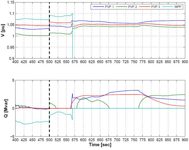
Figure 85: V and Q of all ReGen plants when subject to a cyber-attack (manipulating voltage setpoint at t = 500 s)
