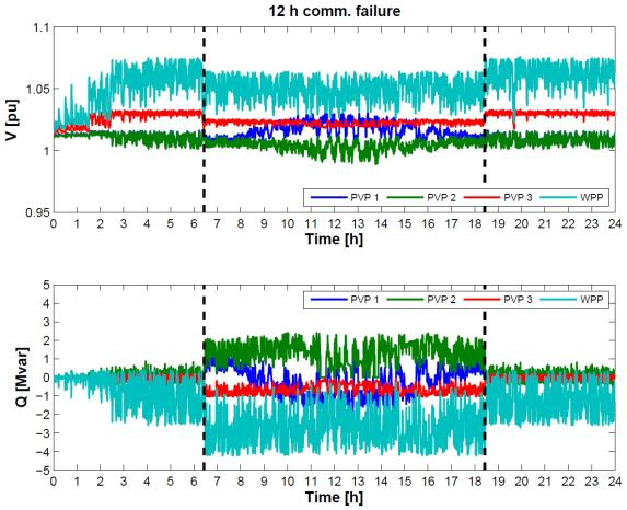
Figure 83: V and Q of all ReGen plants over one day for a communication failure occuring between 6 am and 6 pm
