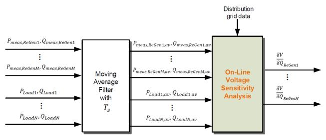
Figure 63: Scheme for on-line voltage sensitivity analysis
