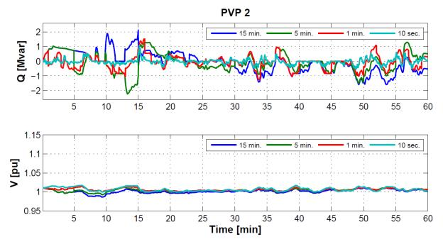
Figure 68: Q and V of PVP 2 over one hour for various update rates Ts for voltage setpoint and grid voltage of  $V_{grid} = 1.00 \ pu$
