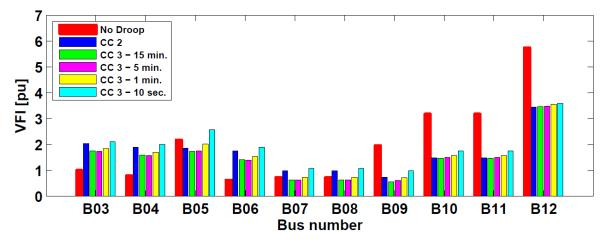
Figure 72: VFI for all MV busses and various various update rates for the voltage setpoint and grid voltage of  $V_{artd} = 1.00 \, pu$
