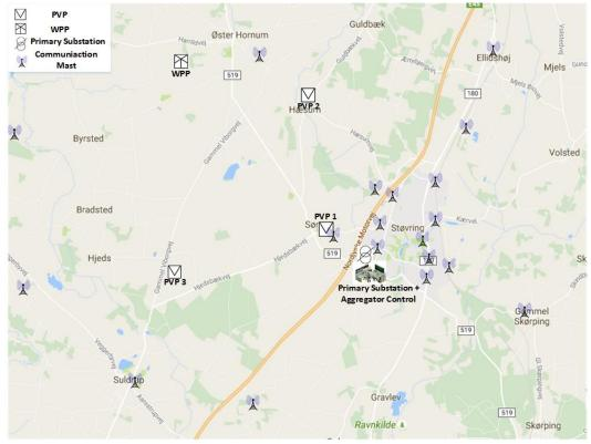
Figure 77: Concept of communication approach when aggregator is placed in local primary substation
