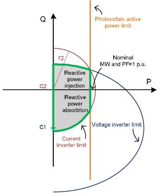
Figure 58: Active and reactive power capacity of PV generator [36]
