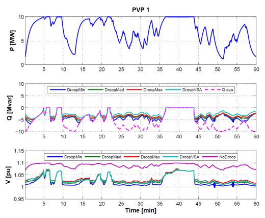
Figure 47: P, Q, V of PVP 1 over one hour for different droop settings and grid voltage of  $V_{grid}=$  1.05 pu
