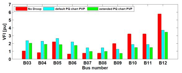
Figure 59: VFI for all MV busses and various PQ charts of PVP and grid voltage of  $V_{arid} = 1.00 \ pu$
