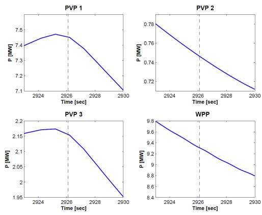
Figure 52: P of all plants at beginning of instability at t1= 48.75 min = 2926.1 sec for DroopMin = 2 %
