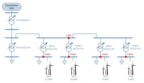
Figure 2: Simplified Single Line Diagram of a 150 kV substation
