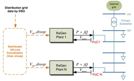
Figure 36: Scheme of control concept 2 - Distributed Off-Line Coordination
