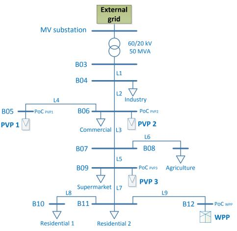
Figure 12: Structure of MV Benchmark Grid
