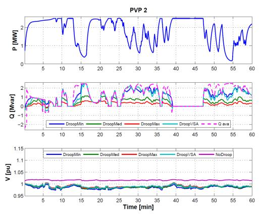
Figure 42: P, Q, V of PVP 2 over one hour for different droop settings and grid voltage of  $V_{grid}=1.00\ pu$
