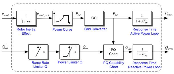
Figure 13: Block diagram of wind power module
