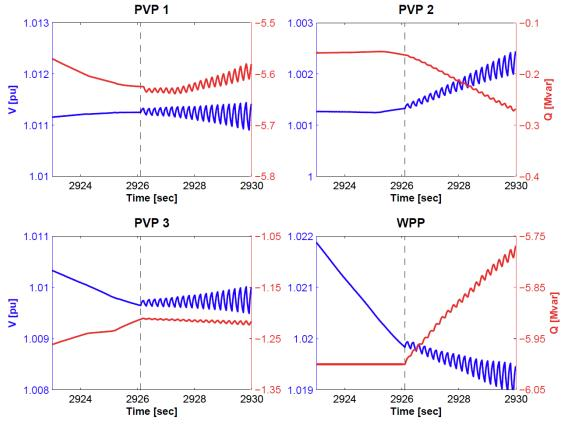
Figure 51: V & Q of all plants at beginning of instability at t1= 48.75 min = 2926.1 sec for DroopMin = 2 %
