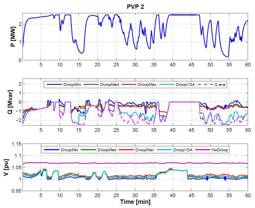
Figure 48: P, Q, V of PVP 2 over one hour for different droop settings and grid voltage of  $V_{grid}=1.05\ pu$
