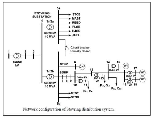
Figure 11: Primary Substation and MV feeder configuration from HEF grid [21]
