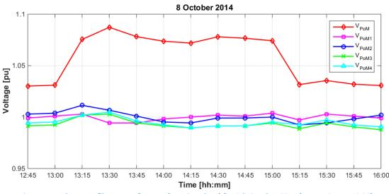
Figure 5. : Voltage profile at transformers (15 min values) for 8th October 2014 (zoom 12:45 – 16:00)
