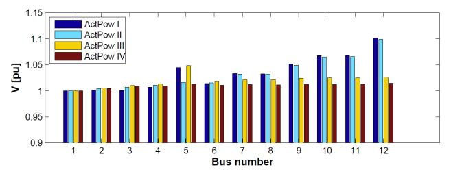
Figure 24: Voltage profile for various operational points of ReGen plants
