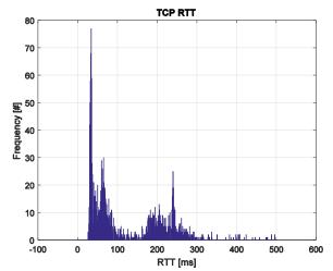
Figure 80: Distribution of TCP RTT measured around the benchmark region
