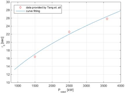
Figure 14: Natural time constant for given rated output of WT [23]
