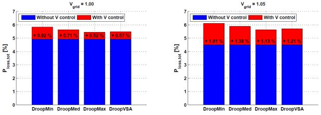
Figure 56: Power losses within the distribution grid for various droop settings (left:  $V_{grid} = 1.00 \, pu$ , right:  $V_{grid} = 1.05 \, pu$ )
