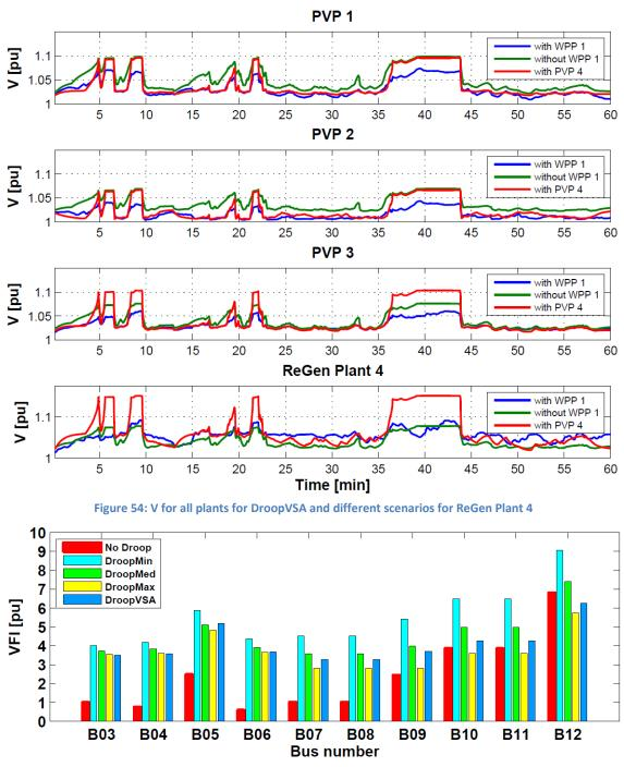
Figure 55: VFI for all MV busses and various droop settings and grid voltage of  $V_{grid} = 1.05 \ pu$
