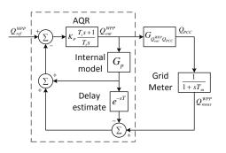
Figure 6. Extended control structure of wind power plant AQR with *Smith Predictor*
