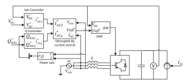
Figure 2. Schematic diagram of grid-side converter and its controller for a type-4 WT.
