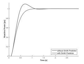
Figure 7. Reactive power step response of closed-loop system with wind power plant AQR with and without *Smith Predictor* for  $t_d = 0.1 \text{ s}$
