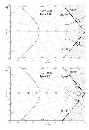
Figure 11. Root locus plots of AVR open-loop system with  $SCR_{min}$  and slope of 4 %: a) with  $T_{PO} = 0.22 \text{ s}$ , b) with  $T_{PO} = 0.6 \text{ s}$
