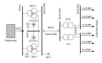
Figure 1. Single line diagram of benchmark offshore wind power plant
