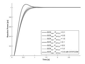
Figure 8. Reactive power step response of closed-loop system with wind power plant AQR including *Smith Predictor* for  $t_d = 0.1 \, \text{s}$  and various test cases
