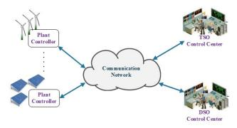
Fig. 1. Communication architecture where several plant controllers are shown communicating with control centers at different levels
