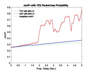
Fig. 6. Mismatch probability versus propagation delay with 95% confidence interval at PER of 10%
