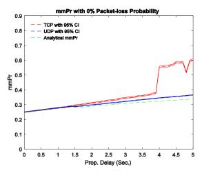
Fig. 5. Mismatch probability versus propagation delay with 95% confidence interval PER of 0%
