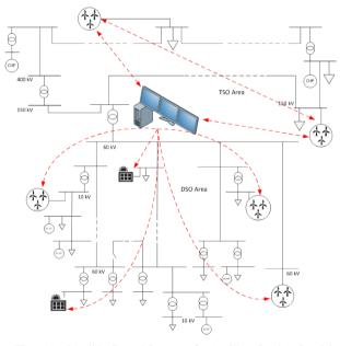
Figure 4. Possible Control Structure for Ancillary Services Provision from Wind and PV Plants in the RePlan Project
